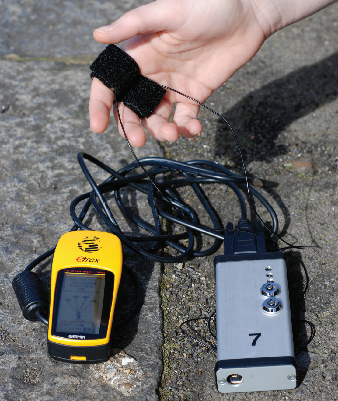
The Bio Mapping device: GPS – left, fingercuffs – top and data logger on the right.
