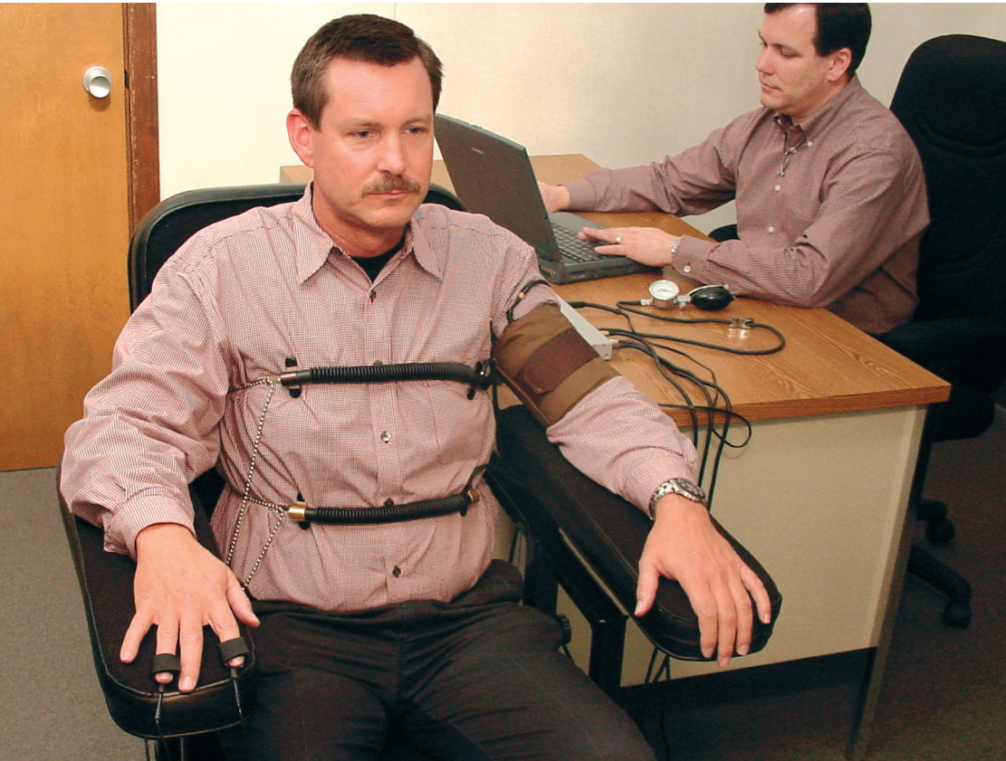
A modern lie detector, combining sensors for breathing rate across the chest, blood pressure on the arm and galvanic skin response on the fingers.
